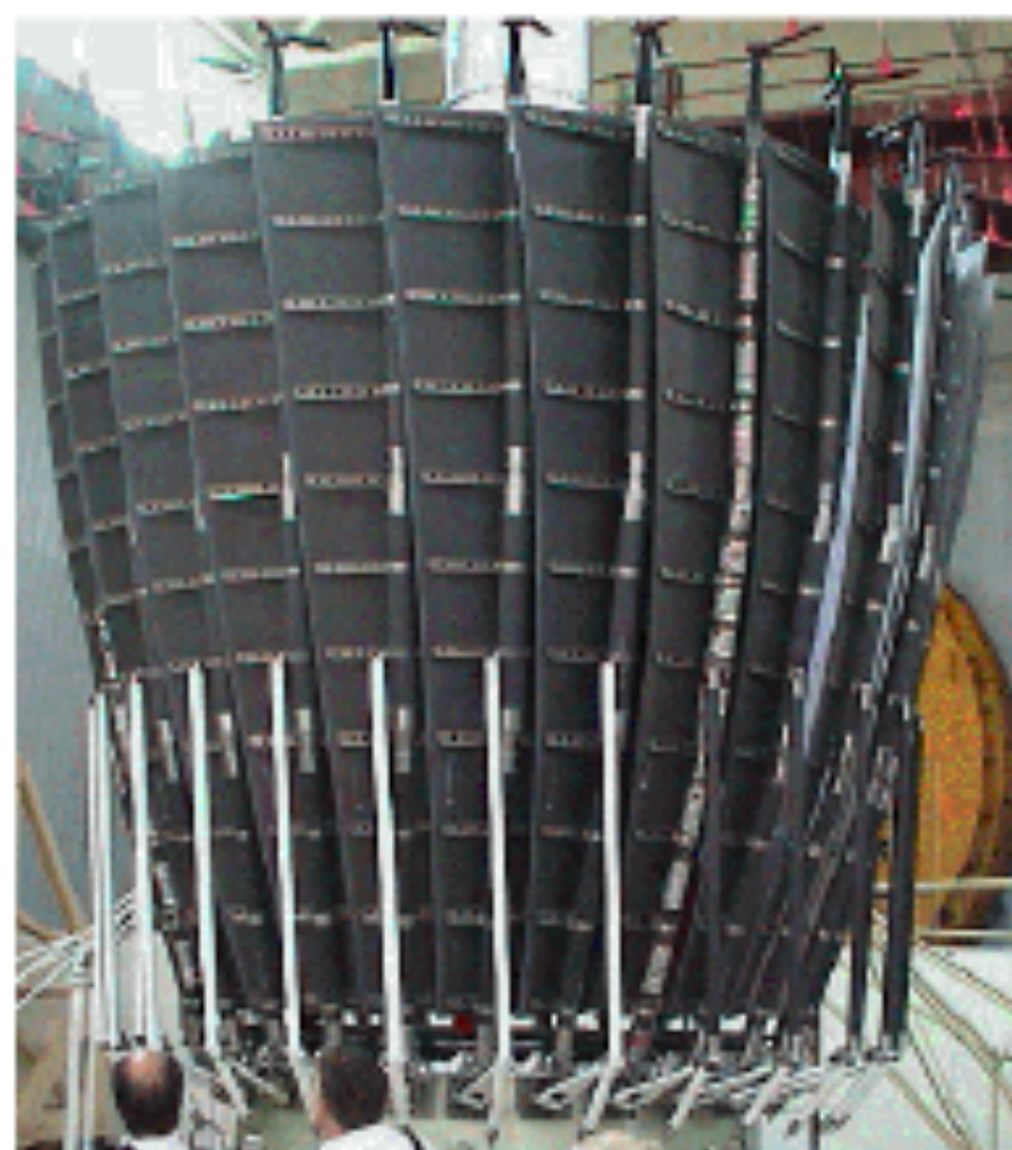
Fig. 9. Radioastron reflector by Lavochkin
